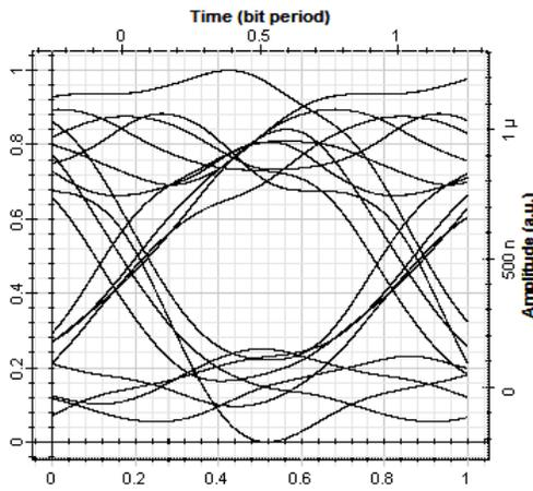
Fig 16: Eye diagram at -124 dBm input laser power for NRZ format
